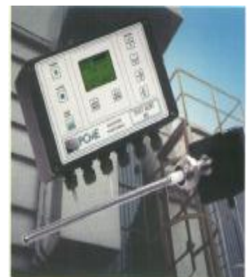
Figure 2 : Photographs of bagfilters on Sinter plant and shotblasting applications with Electrodynamic instrument superimposed.
